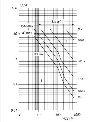
Fig.10. Forward bias safe operating area.  $T_{hs} = 25^{\circ}C$  | Region of permissible DC operation. | Extension for repetitive pulse operation.
