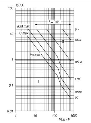
Fig.11. Forward bias safe operating area.  $T_{hs} = 25^{\circ}C$  I Region of permissible DC operation. II Extension for repetitive pulse operation.
