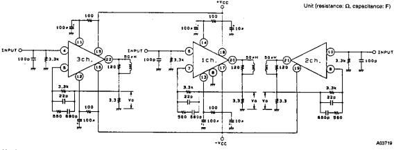
Vo:  $V_{NO}$  is measured by connecting a VTVM.  $V_{N}$  is measured by connecting a DC voltmeter.  $t_{D}$  is measured by connecting an oscilloscope.
