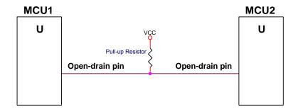
The pull-up resistor is necessary. Open-drain output high is driven by pull-up resistor. Output low is sunken by MCU's pin.
