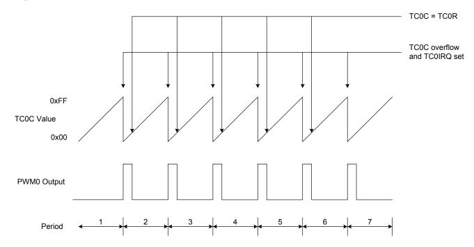
Above diagram is shown the waveform with fixed TC0R. In every TC0C overflow PWM output "High, when TC0C≧ TC0R PWM output "Low". If TC0R is changing in the program processing, the PWM waveform will became as following diagram.
