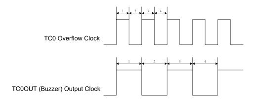
Example: Setup TC0OUT output from TC0 to TC0OUT (P5.4). The external high-speed clock is 4MHz. The TC0OUT frequency is 0.5KHz. Because the TC0OUT signal is divided by 2, set the TC0 clock to 1KHz. The TC0 clock source is from external oscillator clock. T0C rate is Fcpu/4. The TC0RATE2~TC0RATE1 = 110. TC0C = TC0R = 131.
