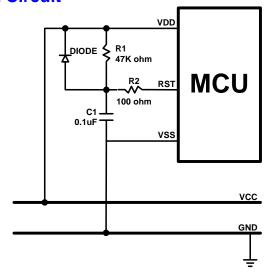
This is the better reset circuit. The R1 and C1 circuit operation is like the simply reset circuit to make a power on signal. The reset circuit has a simply protection against unusual power. The diode offers a power positive path to conduct higher power to VDD. It is can make reset pin voltage level to synchronize with VDD voltage. The structure can improve slight brown out reset condition.
