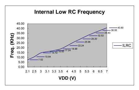
The internal low RC supports watchdog clock source and system slow mode controlled by CLKMD.
