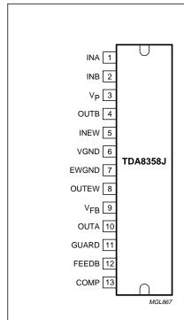
The die has been glued to the metal block of the package. If the metal block is not insulated from the heatsink, the heatsink shall only be connected directly to pin VGND.
