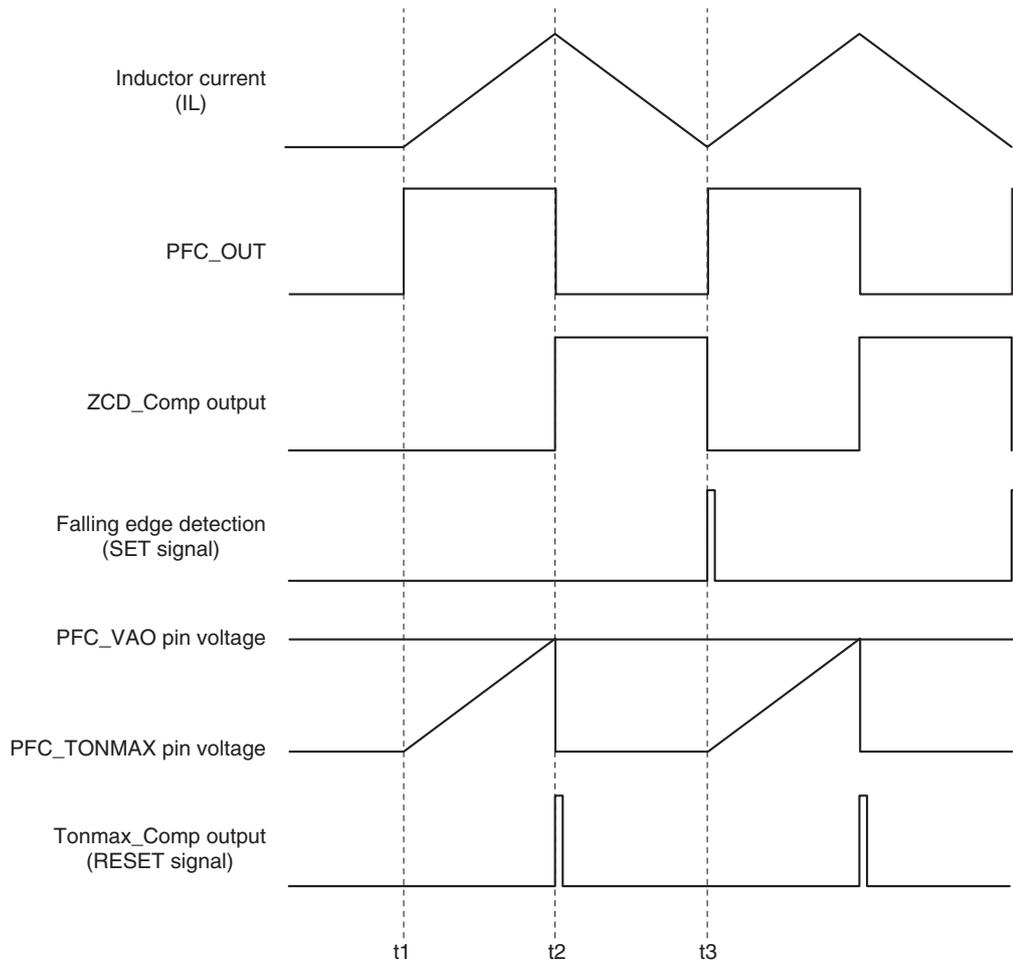
Fig. 6. Switching Operation Block Waveforms
