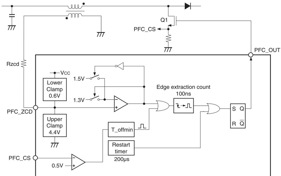
**Fig. 7. ZCD Control Block Equivalent Circuit**
