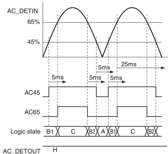
**Fig. 3. AC\_DETIN Input Waveform and State Transitions**
