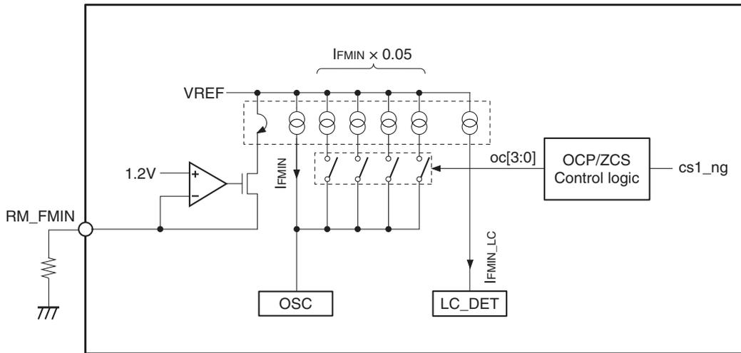
Fig. 13. Minimum Resonant Frequency Control Block Equivalent Circuit
