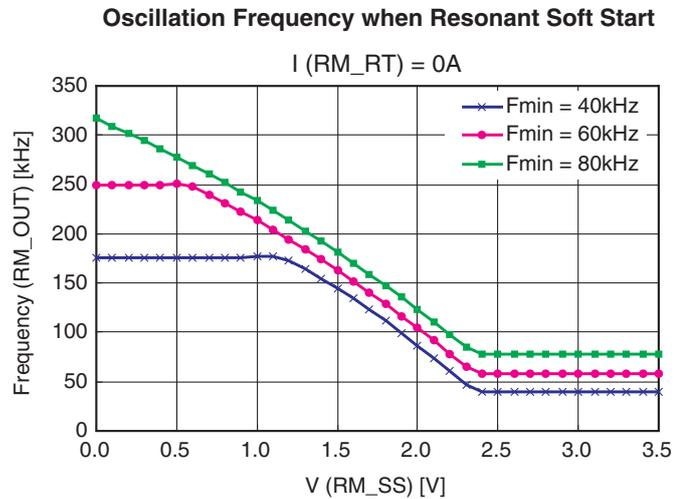
Fig. 16. Resonant Oscillation Frequency during Soft Start
