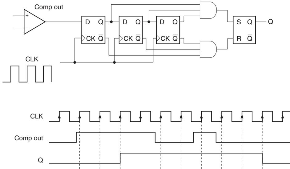
Fig. 1. Equivalent Circuit Corresponded to 1ms × 3 Times
