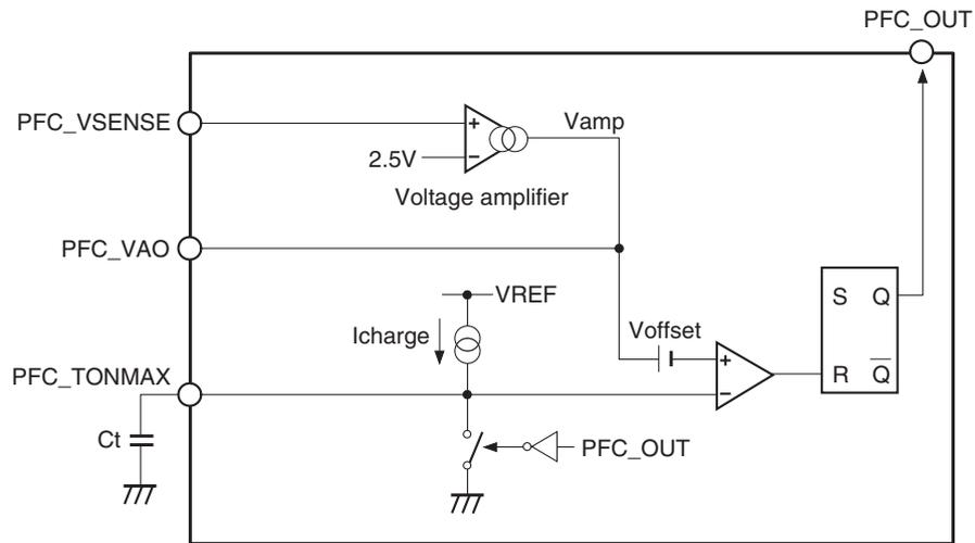
**Fig. 8. Maximum ON Time Control Block Equivalent Circuit**
