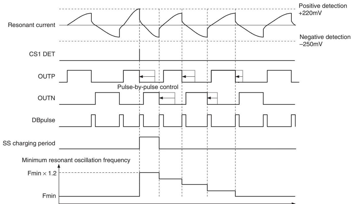
**Fig. 18. Operating Waveform in Overcurrent Detection Mode**
