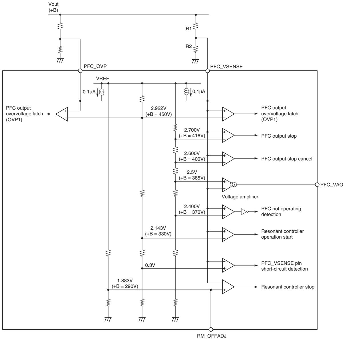
Fig. 10. PFC Output Voltage Detection Block Equivalent Circuit
