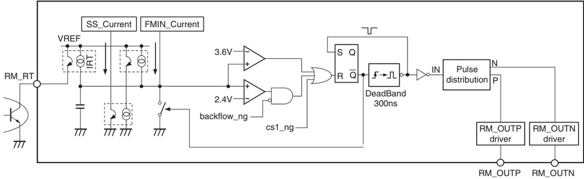
Fig. 11. Resonant Oscillator Equivalent Circuit
