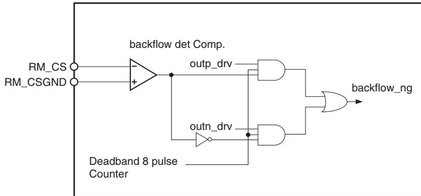
**Fig. 19. Resonant Back Flow Detection Block Equivalent Circuit**
