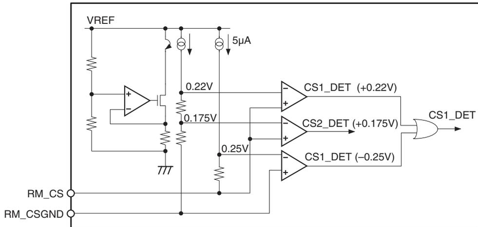
**Fig. 17. Overcurrent Detection Block Equivalent Circuit**
