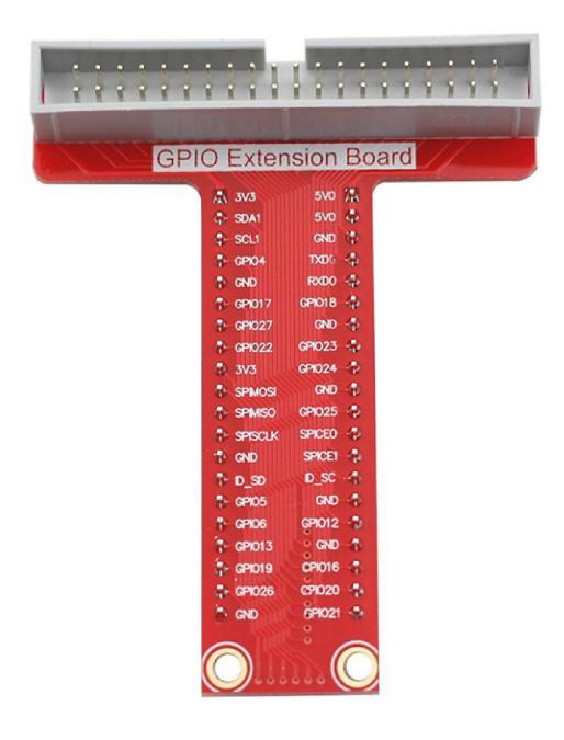
Connected with Raspberry Pi shown below, the principle is lead out the raspberry pi GPIO by GPIO cable to the GPIO pin extension board and extention board inserted into the breadboard, when you jump wire is inserted into the breadboard, equivalent inserted into the raspberry Pi GPIO.
