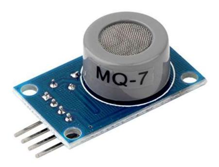
MQ-7 is a highly sensitive gas sensor which is capable of detecting 10 to 10,000 ppm carbon monoxide concentrations in the air. The sensor needs only one analog input of the microprocessor. It is a low cost sensor that is very useful as gas monitoring devices.
