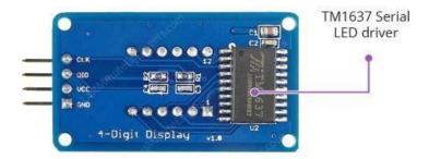
The TM1637 supports many functions – including ON/OFF and brightness control of the LEDs as well as accessing each of the segments. It also allows you to adjust the brightness of the LEDs at software level.
