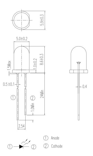
Note: Tolerances unless dimensions ±0.25mm
