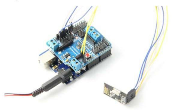
First of all, you need two Arduino boards and at least two RF modules, one to transmit and the other to receive. If you don't have, you can get them in our store in a very low cost. (Order nRF24L01 module)If you use a standard Arduino board, you should use the Arduino board's 3.3V pin to provide power. Beacuse the nRF24L01 module is worked at 1.9-3.6V voltage level.
