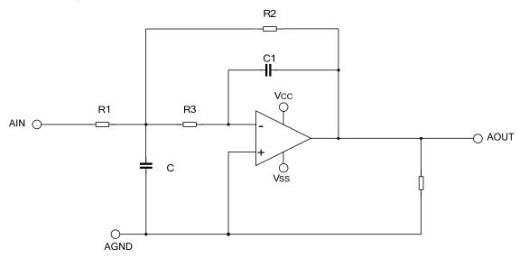
The second-order filter structure shown as above is adopted for 3-channel audio amplifier, with in-band gain of about 12dB and -3dB bandwidth of 40kHz above which is well meet audio requirements. As principle structure, in-band gain is decided by:  $G = -\frac{R_2}{R_1}$ , thus, gain can be adjusted by changing R1.
