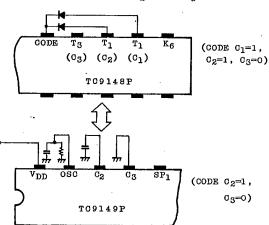
The combination of code bits of TC9148P and TC9149P is shown in Table 1  $\,$
