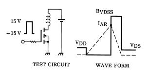
$$\begin{aligned} R_G &= 25~\Omega \\ V_{DD} &= 90~V,~L = 60~mH \end{aligned} \qquad E_{AS} &= \frac{1}{2} \cdot L \cdot I^2 \cdot \left( \frac{BVDSS}{BVDSS - V_{DD}} \right) \end{aligned}$$
