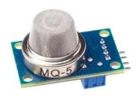
Gas Sensor(MQ5) module is useful for gas leakage detection (in home and industry). It is suitable for detecting H2, LPG, CH4, CO, Alcohol. Due to its high sensitivity and fast response time, measurements can be taken as soon as possible. The sensitivity of the sensor can be adjusted by using the potentiometer.
