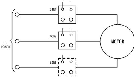
Three-phase motors may be controlled by solid-state relays as shown. A third SSR as shown is optional, but not necessary. The control windings may be connected in series or parallel. Care should be taken to ensure that surge current drawn by the motor does not exceed surge current rating of the SSR.
