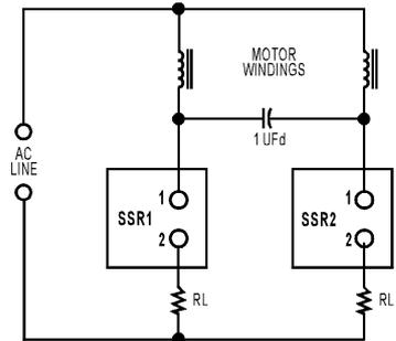
The resistors are unnecessary if the control circuit is designed to ensure one SSR is off before the other SSR is on.
