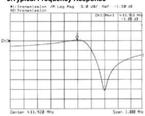
The curve shown above accounts for resonator contribution only and does not include oscillator temperature characteristics.
